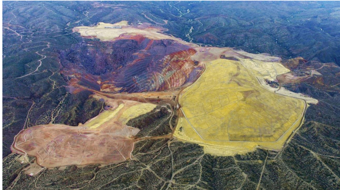
Copper mine in Arizona regraded and recontoured with planting for revegetation
